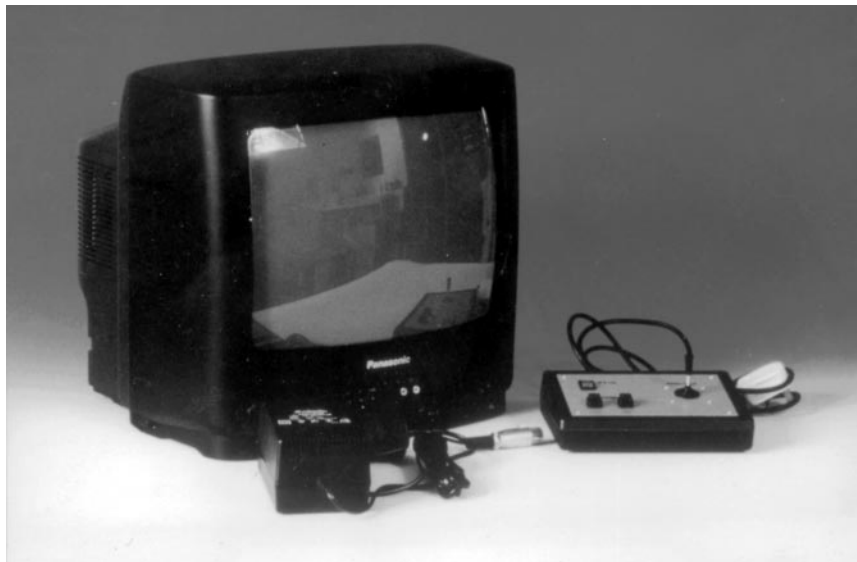
Figure 2 The video monitor and the remote pan/tilt/zoom control unit.
